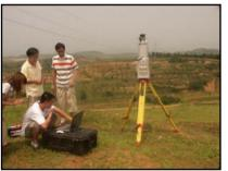
Lidar survey of digital elevation model (DEM)
